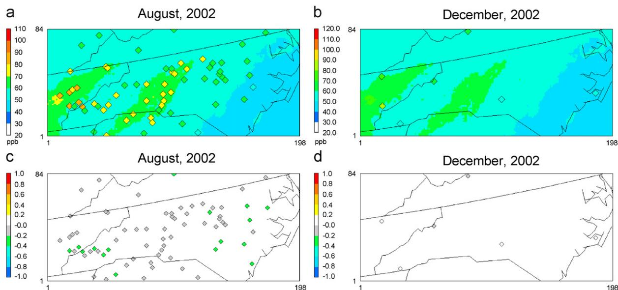
Fig. 5. The overlay of simulated and observed spatial distributions of monthly mean 1-h maximum  $\text{O}_3$  mixing ratios (a) and (b) along with NMBs (c) and (d). The observational datasets are taken from AQS and CASTNet in August and December, and from CASTNet only for December.
