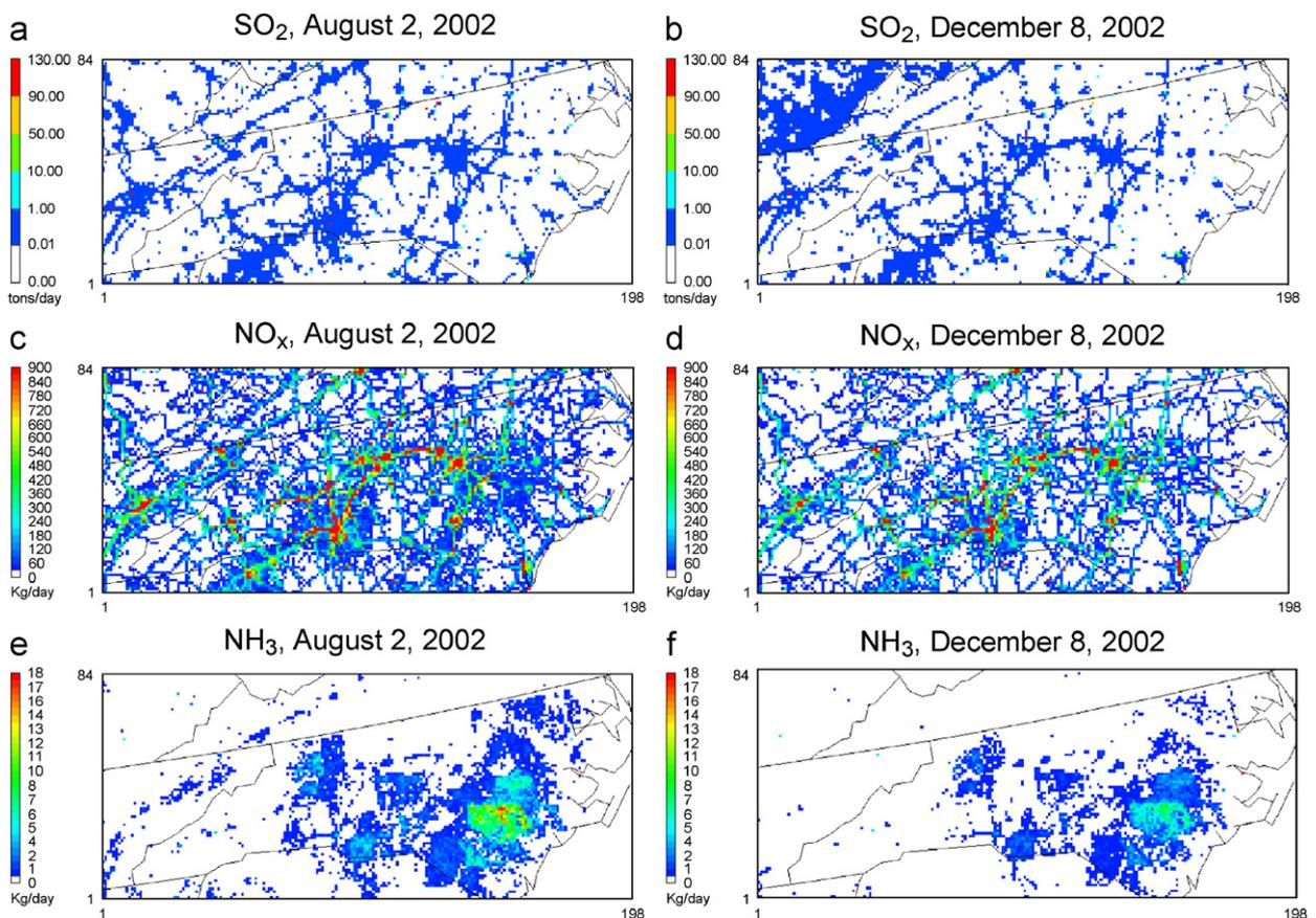
Fig. 2. The daily total emissions of  $\text{SO}_2$  (a) and (b),  $\text{NO}_x$  (c) and (d), and  $\text{NH}_3$  (e) and (f) for the 4-km simulation (generated using raw emission inventories from VISTAS).
