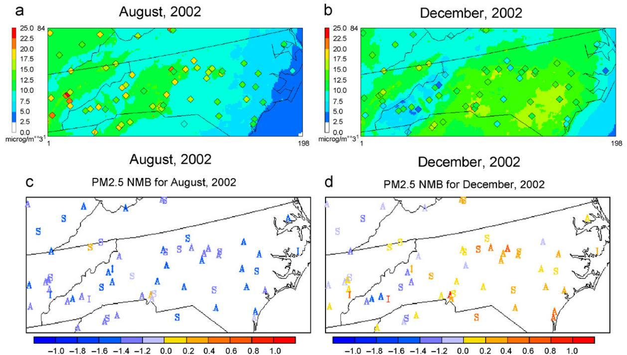
Fig. 6. The overlay of simulated and observed spatial distributions of monthly mean 24-h average PM<sub>2.5</sub> concentrations (a) and (b) along with NMBs (c) and (d). The observational datasets are taken from AQS, STN, and IMPROVE networks for both months.
