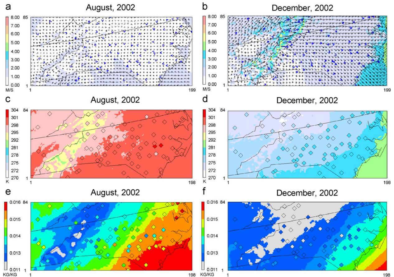
Fig. 3. Observed and simulated monthly-mean surface wind vectors at 10 and 19 m, respectively (a) and (b), monthly-mean surface temperatures at 2-m (c) and (d), and water vapor mixing ratios at 2-m (e) and (f). The diamonds indicate observed values.
