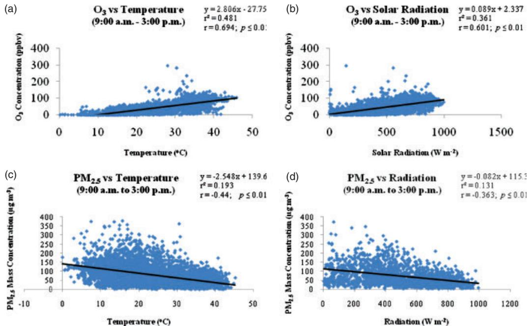
Figure 10. Correlation of ozone and  $PM_{2.5}$  with temperature and solar radiation variables during 2007–2011 at 9:00 A.M. to 3:00 P.M.
