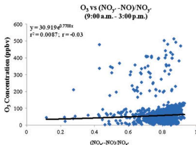
**Figure 8.** Variation of concentration of ozone vs.  $(\text{NO}_y - \text{NO})/\text{NO}_y$  in the summer months for 2007–2011 during maximum photochemical activity of the day, i.e., 9:00 A.M. to 3:00 P.M.
