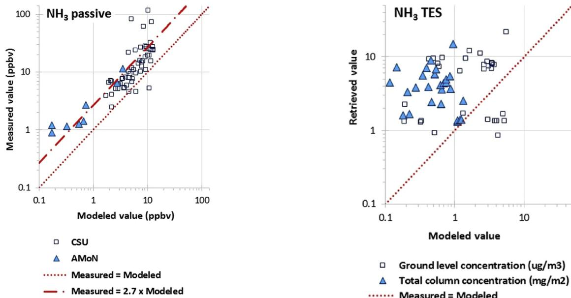
**Fig. 5.** Ground-level measurements of NH<sub>3</sub> plotted against model predictions. Dotted line shows where the measured points should have fallen if the model predictions were exactly correct (measured = modeled). Dashed line shows the actual measured trend lines based on the ratio of the average measured concentration to the average model prediction.
