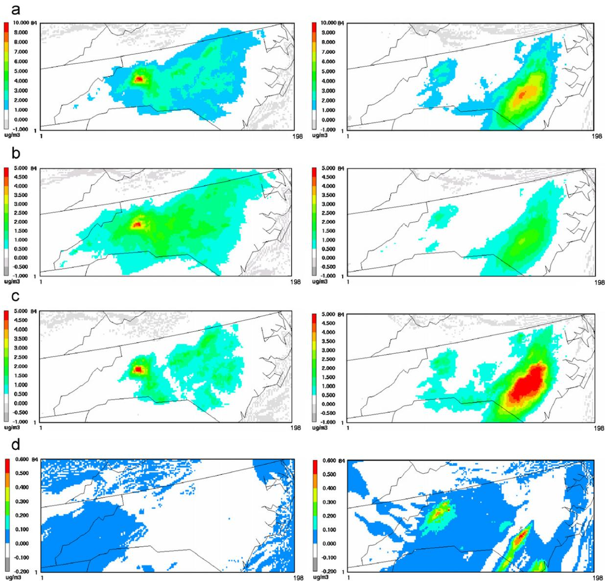
Fig. 3. The contribution of AL-NH<sub>3</sub> emissions to daily average concentrations of (a) PM<sub>2.5</sub>, (b) NH<sub>4</sub><sup>+</sup>, (c) NO<sub>3</sub><sup>-</sup>, and (d) SO<sub>4</sub><sup>2-</sup> on 2 August (left) and 31 August (right) 2002.
