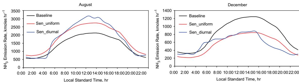
Fig. 1. NH<sub>3</sub> emission profiles used in the baseline and sensitivity simulations.
