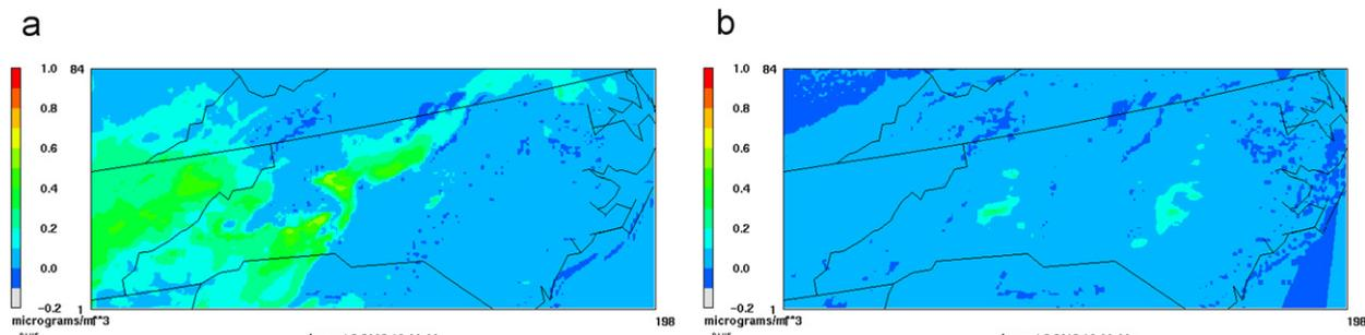
Fig. 7. Changes in the concentrations of (a)  $\text{NH}_4^+$  and (b)  $\text{NO}_3^-$  due to emission adjustments in Sen\_uniform at 11 a.m. EST 2 August 2002.
