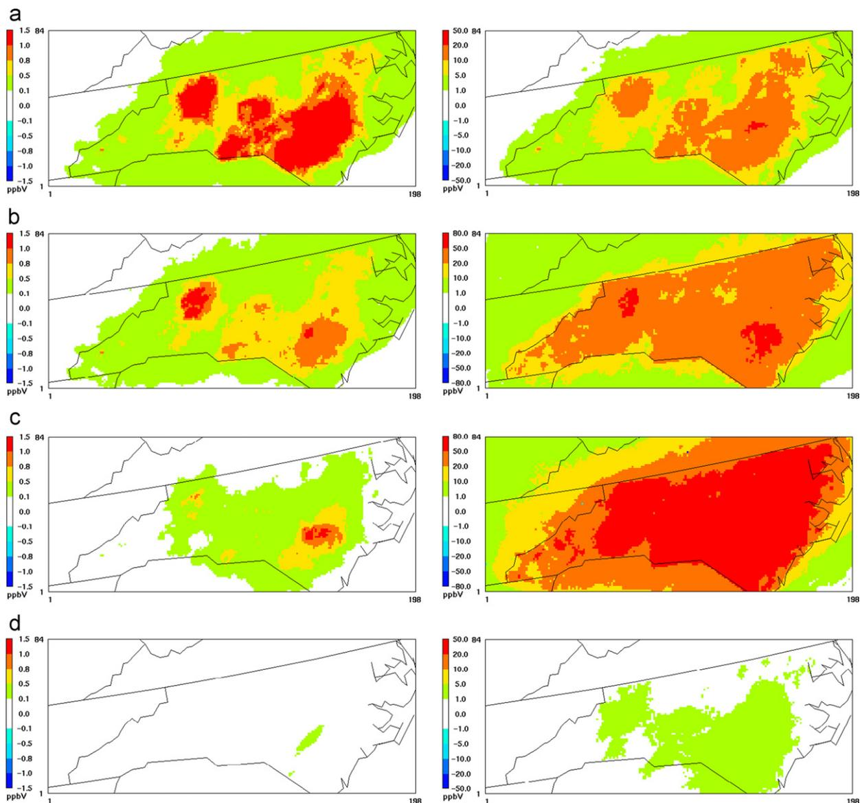
Fig. 2. The monthly mean contributions of AL-NH<sub>3</sub> emissions to (a) PM<sub>2.5</sub>, (b) NH<sub>4</sub><sup>+</sup>, (c) NO<sub>3</sub><sup>-</sup>, and (d) SO<sub>4</sub><sup>2-</sup> in term of absolute (left) and percent (right) changes in August 2002.
