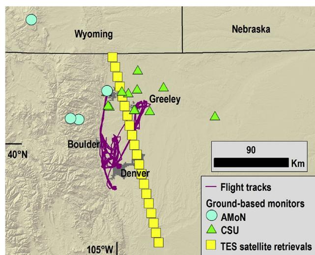
Fig. 1. Domain of the DISCOVER-AQ Colorado measurement campaign, showing flight paths for low level *in situ* aircraft measurements (<1 km AGL), locations of ground level monitors, and the path for TES satellite measurements.
