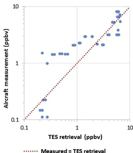
**Fig. 7.** Aircraft *in situ* measurements of NH<sub>3</sub> plotted against TES satellite retrievals. Each measurement is plotted as a point. Dotted line shows where the measured points should have fallen if the satellite retrievals were exactly correct (measured = TES retrieval).
