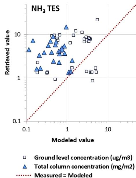
**Fig. 5.** Ground-level measurements of NH<sub>3</sub> plotted against model predictions. Dotted line shows where the measured points should have fallen if the model predictions were exactly correct (measured = modeled). Dashed line shows the actual measured trend lines based on the ratio of the average measured concentration to the average model prediction.
