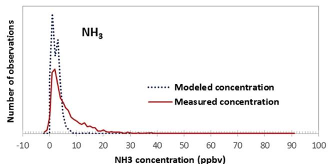
**Fig. 3.** Histogram of aircraft measurements compared with histogram of model predictions at the corresponding times and locations.
