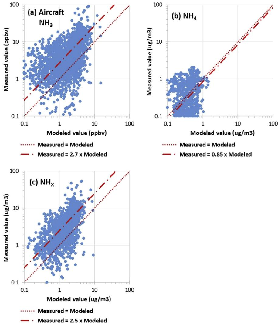
**Fig. 2.** Aircraft *in situ* measurements of  $\text{NH}_3$  (a),  $\text{NH}_4^+$  (b), and  $\text{NH}_x$  (c), plotted against model predictions. Each measurement is plotted as a point. Dotted lines show a 1:1 slope, where points would have fallen if the measurements and model predictions were in complete agreement (measured = modeled). Dashed lines show the 1:1 slope displaced by the NMB.
