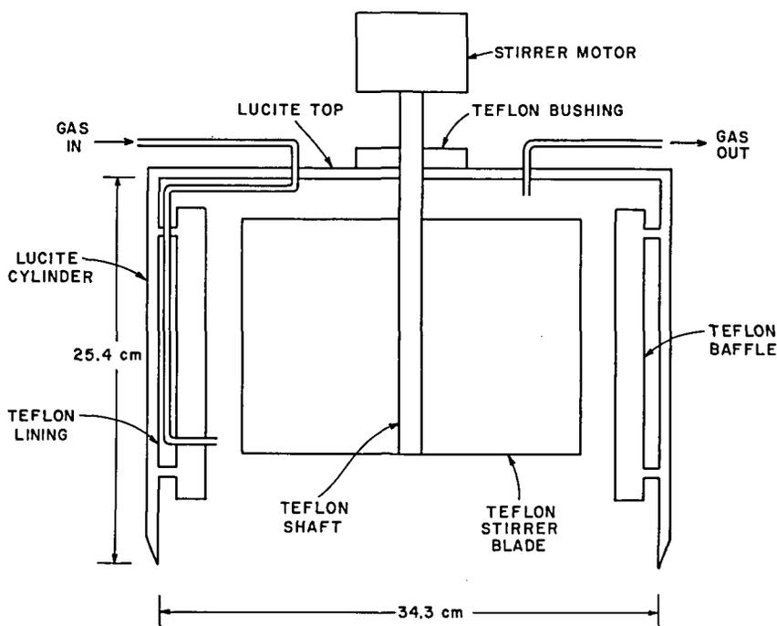
FIG. 2 Emission flux chamber used at Flax Pond, Old Field, N. Y.
