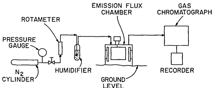
FIG. 3 Apparatus used at Flax Pond, Old Field, N. Y.
